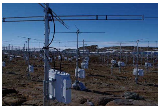
Figure 1. TR modules and antenna elements of PANSY radar constructed at Syowa station.
