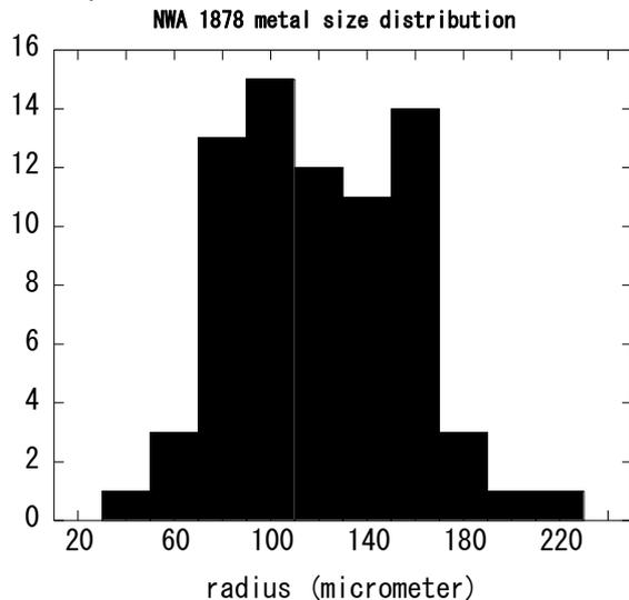
Fig.2 Grain size distribution of metals seen in Fig.1. The radius is that of a sphere with an area equal to the fitted spheroid.
