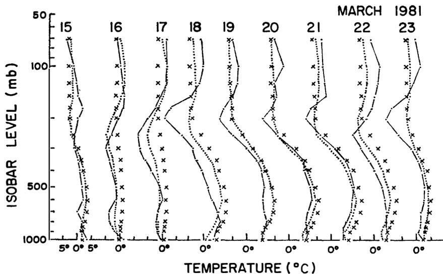
Fig. 1. A successive day-to-day pattern of vertical profiles of temperature. Solid and dotted lines show the observed and the estimated profiles, respectively, where cross marks are for the hard muon analysis. All values of temperature are deviations from the common profile averaged over the period from November 1980 to March 1981.
