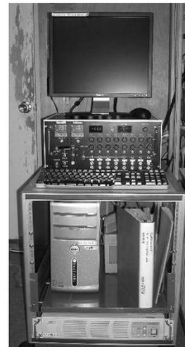
Fig. 1. Photos of the 8 color meridian scanning photometer at Syowa Station.
