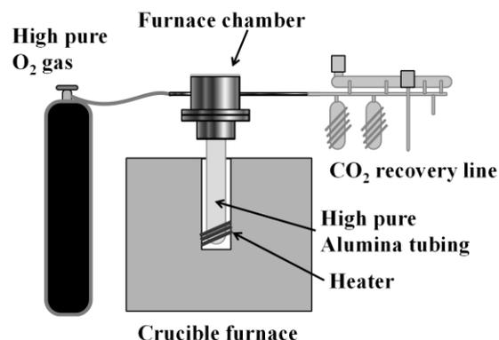
Figure 1. The extremely low level  $^{14}\text{C}$  extraction system for HED meteorites at Rissho University
