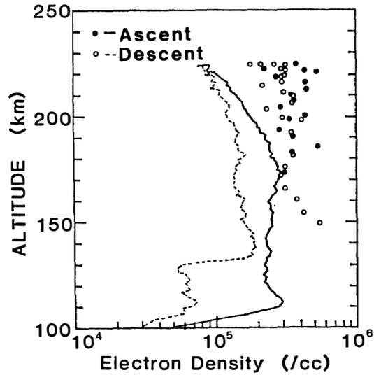
Fig. 4. The calculated (circles) and observed (curves, after T. TAKAHASHI) electron density as a function of altitude in the S-310JA-5 rocket experiment.
