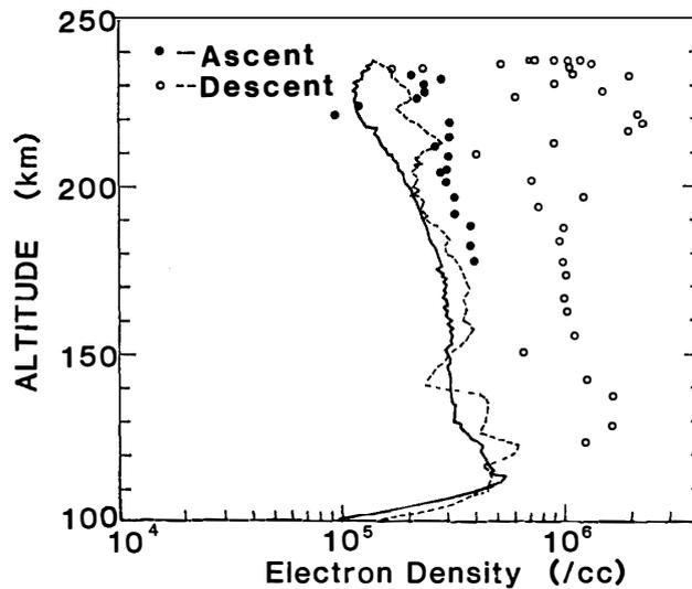
Fig. 5. The calculated (circles) and observed (curves, after T. TAKAHASHI) electron density as a function of altitude in the S-310JA-6 rocket experiment.
