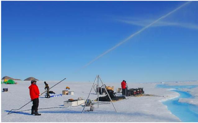
Figure 1. Hot water drilling on Langhovde Glacier, Antarctica.
