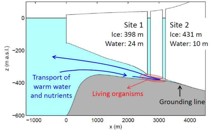
Figure 2. Cross section of Langhovde Glacier as revealed by the drilling.
