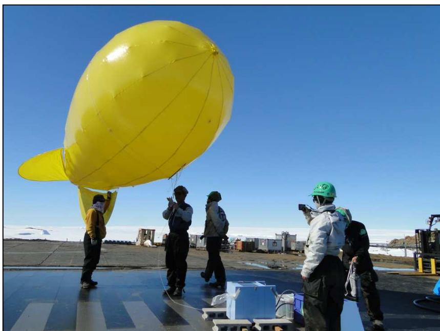
Figure 1. The sampling of atmospheric bioaerosol using a tethered balloon (Photo by Inai).
