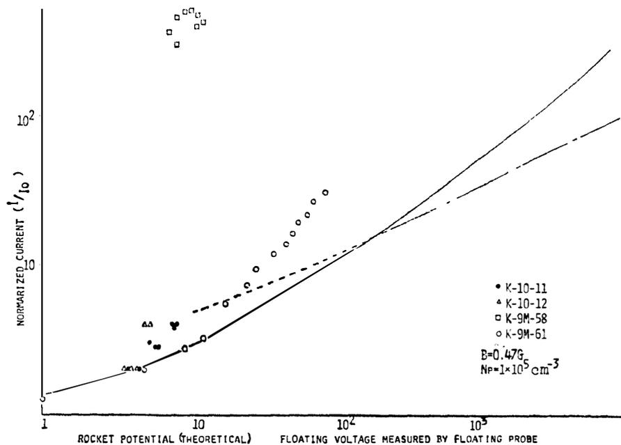
Fig. 2. Summary of the floating probe data in the rocket experiments. The solid line shows the theoretical model of BEARD and JOHNSON. The experimental data depart from the line as the beam current increases because a considerable amount of plasma is produced surrounding the rocket body.
