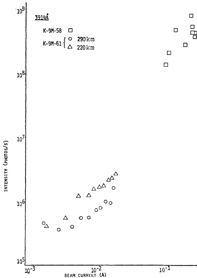
Fig. 5. Intensity of 3914 Å in K-9M-58 and in K-9M-61 experiment as a function of the beam current. Photon intensity of  $10^{10}$  photons/s  $\text{cm}^2$  is expected in the high-power electron beam experiment.
