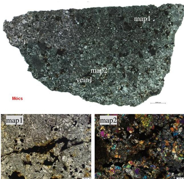
Figure 1: Stereomicroscopic image of thin section of Mόcs meteorite marked with the measuring areas. Optical microscopic photos of area map1 (plain polarized light) and map2 (crossed polars)
