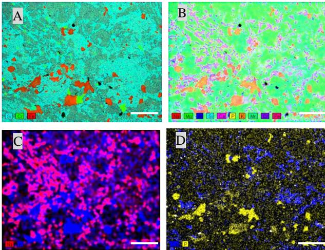
Fig. 2. Composite element maps of upper part in shock vein (map 1 in Fig. 1.) including chondrule fragments (A: Si-Cr-Fe, B: composite element map of major elements and Cr, C: Na-K, D: Ca-P, scale: 200  $\mu\text{m}$ )
