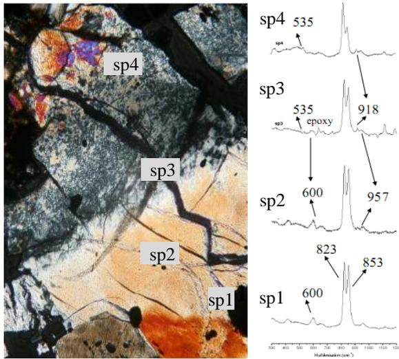
Fig. 2: Raman spectra of differently shocked olivine.
