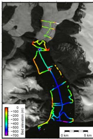
Figure 2. Glacier and ocean bed elevation measured in the field.
