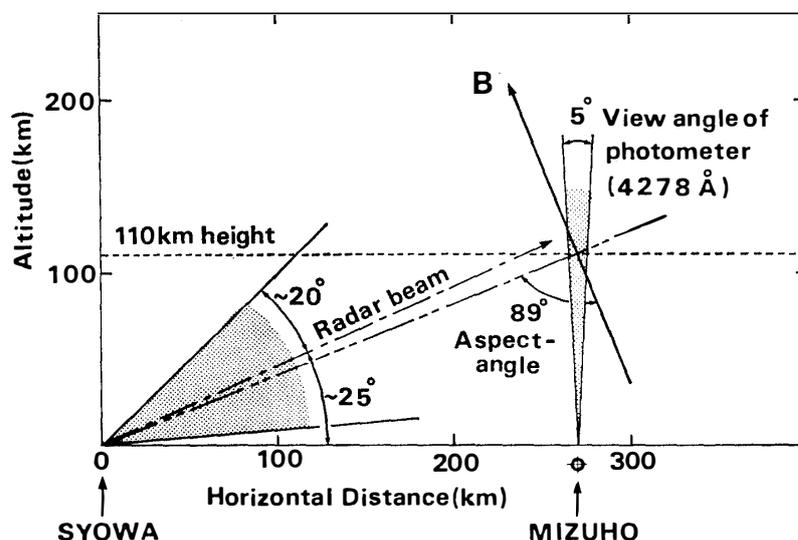
Fig. 2. Locations of the photometer and the region observed by the auroral radar. The elevation angle of the radar is  $25^\circ$ , the half-power beam width of the radar is about  $40^\circ$ , and the view angle of the photometer is  $5^\circ$ .
