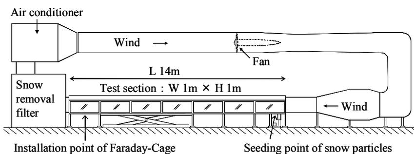
Fig.2 Schematic of wind tunnel
