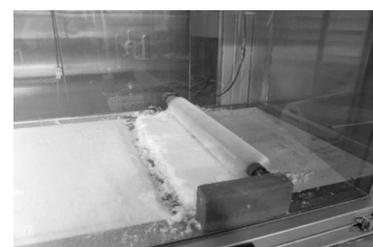
Fig.4 Automatic particle seeder
