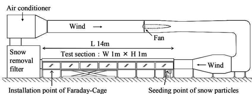
Fig.2 Schematic of wind tunnel
