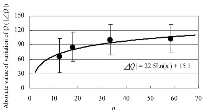
Fig.8 Absolute value of variation of  $Q$  against  $n$ . (Case of spherical particles,  $-20^\circ\text{C}$ )
