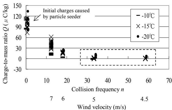
Fig.6 Charge-to-mass ratio  $Q$  against the collision frequency  $n$ . (Case of spherical particles)
