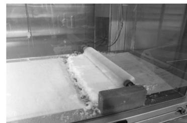
Fig.4 Automatic particle seeder
