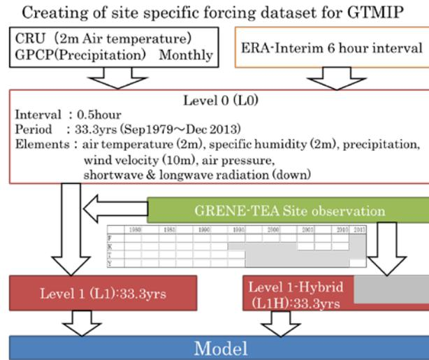
Fig. 2: Schematic diagram of the method for creating the site specific forcing dataset for GTMIP
