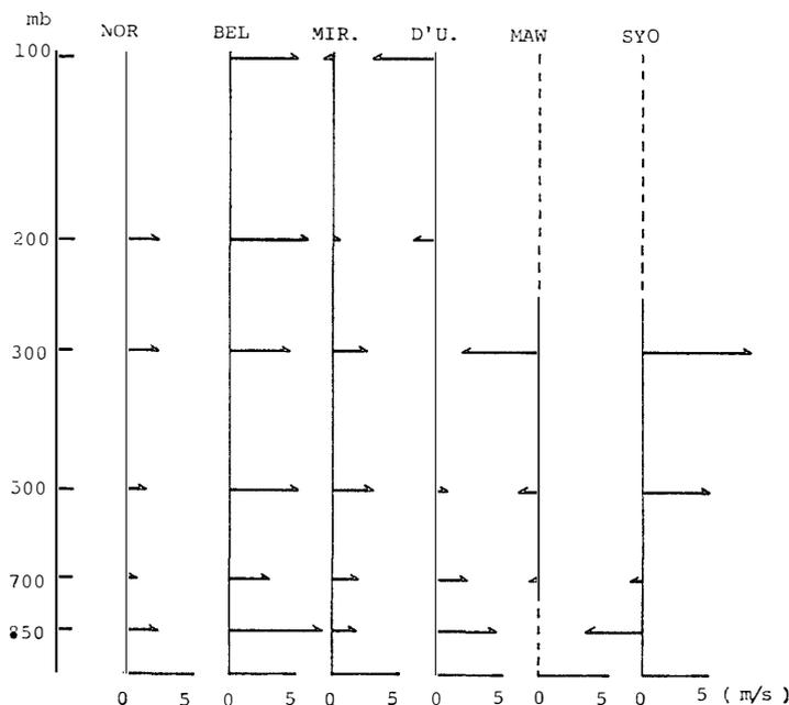
Fig. 4 Mean meridional wind over the East Antarctic coastal stations for June 1958 except Syowa Station (JAPAN METEOROLOGICAL AGENCY, 1976) Positive sign shows outflow from the continent Negative shows inflow. For the location of each station see Fig. 3
