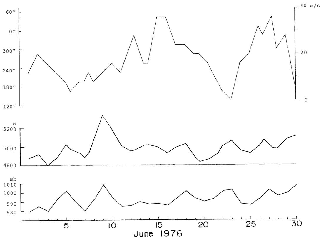
Fig 8 Above Wind direction (solid line) shown by the scale on the left side and wind speed (dotted line) shown by the scale on the right side on the 500 mb surface over Syowa in June 1976 Middle Height of 500 mb surface Below Sea level pressure
