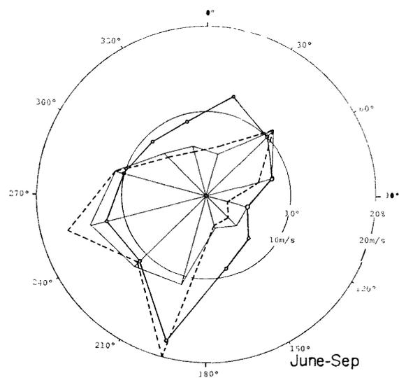
Fig 6 The frequency distribution of wind direction (solid line linking the radial solid line from the center), wind speed (solid line linking the black circle) with direction distinction of  $30^{\circ}$  interval on the 500 mb surface over Syowa Station for June to September 1976. The scale of inner circle shows 10% and 10 m/s. Outer circle 20% and 20 m/s. For the broken line see text.
