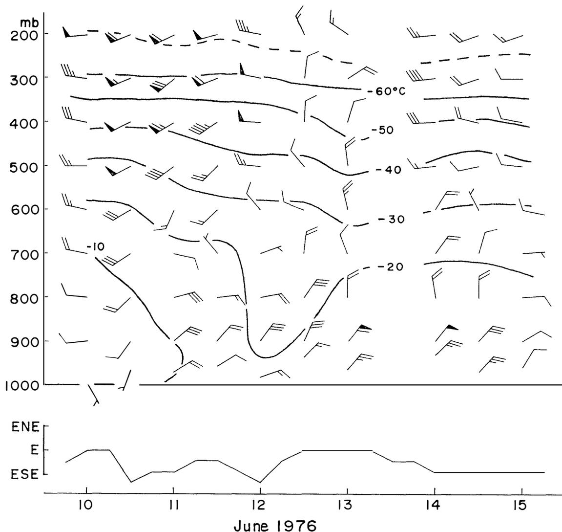
Fig 9. Above: Time section of wind and temperature aloft over Syowa from June 10th 00Z to 15th 00Z, 1976. The broken line shows tropopause. Below. Surface wind direction at Mizuho Station during the same period
