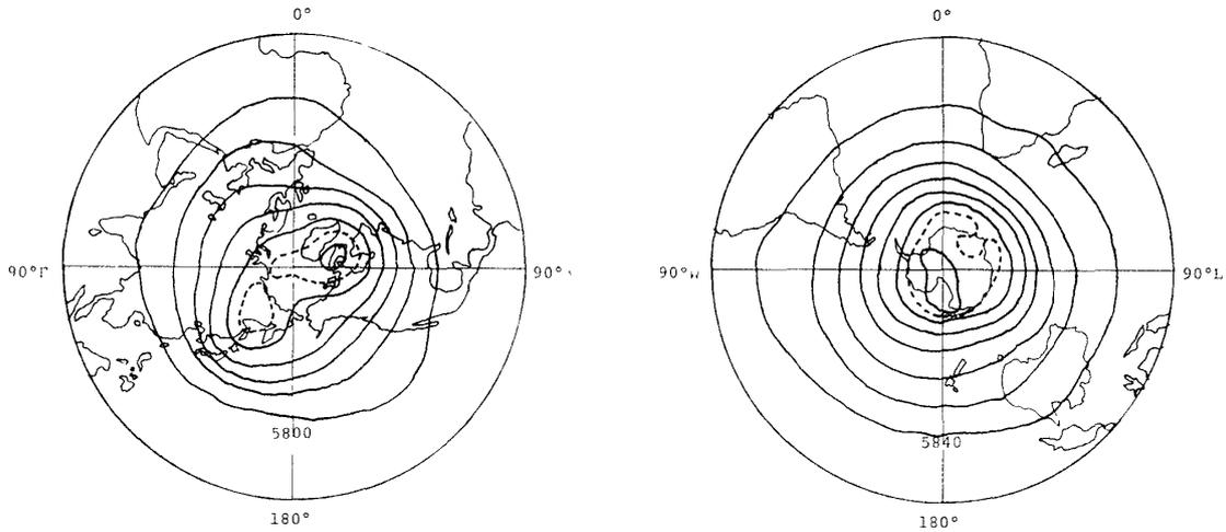
Fig 1 Mean winter 500 mb charts Left Northern hemisphere for January Right Southern hemisphere for July Redrawn from PALMEN and NEWTON's text (1969) with contour interval of 16 gpm
