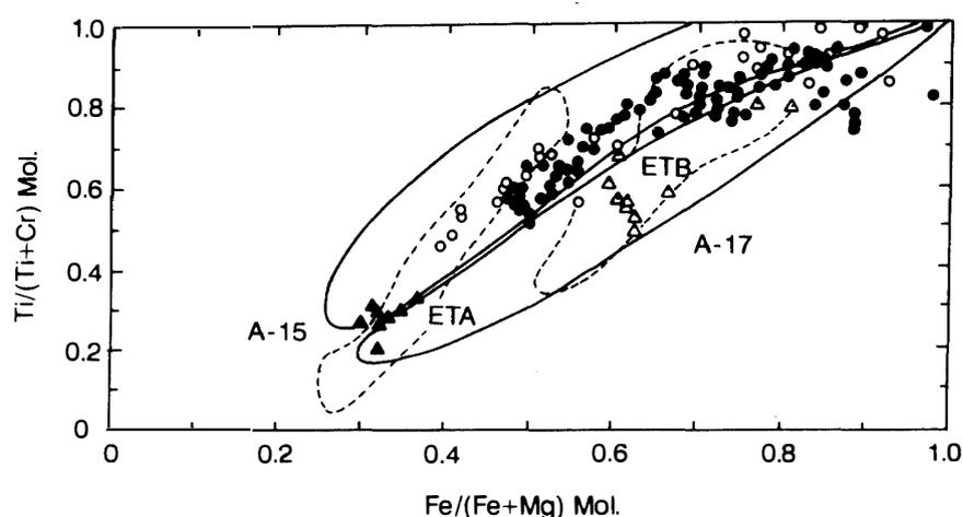
Fig. 5.  $Ti/(Ti+Cr)$  vs.  $Fe/(Fe+Mg)$  mol ratios for pyroxenes in Y-793169. Data from A-15 mare basalts and A-17 VLT basalts are from NIELSEN and DRAKE (1978). Open circles: Y-793169; solid circles: A-881757. ETA and ETB represent Groups A and B of EET87521 (BOESENBERG and DELANEY, 1992). Triangles (filled: Mg-rich and open: Fe-rich): Our data of EET87521.
