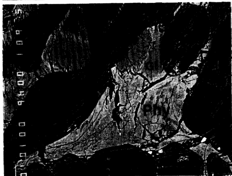
Fig. 1-3. BSE image of the core of a large magnesian chondrule, including coarse-grained olivine (Ol) and enstatite (En), fine-grained diopside (Di), and phyllosilicate (Phy). Glass (Gl) occurs in intimate association with phyllosilicate. Width of 160 microns.
