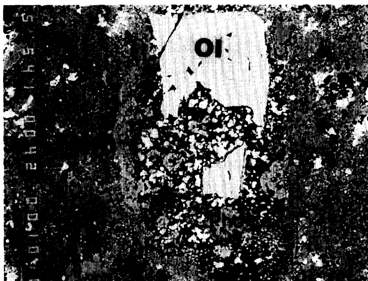
Fig. 1-21. BSE image of a hortonolite-rich clast, consisting of olivine (Ol), kamacite (Kam), and phosphate (Pho). There are abundant cavities, especially around kamacite, in this clast. A phosphate-rich rim surrounds this clast. Width of 170 microns.
