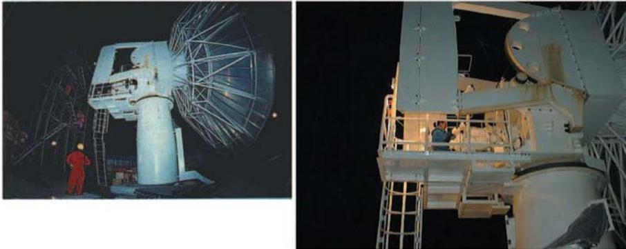
*Antenna overview:* (Left) The antenna is covered with a 17-m diameter radome. (Right) Close-up of the center-hub. There are two pairs of motors to control vertical (elevation) movement and horizontal (azimuth) movement of the 11-m reflector.
