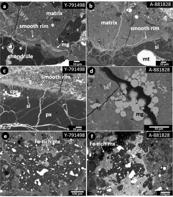
Fig.1. BSE images of characteristic regions of Y-791498 and A-881828. (a, b) Smooth rims around chondrules. Some rims are decorated with fine-grained magnetite grains. Si=silica, mt=Fe-Ni metal. (c) "Honeycomb" structure in high-Ca pyroxene (cpx) rim around chondrule in Y-791498. (d) Framboidal magnetite (mg) are rarely found in A-881828. (e, f) Fe-rich matrix (Fe-rich mx) is characterized by bright regions with Fe-oxides and Fe-sulfides (Fe-sf).
