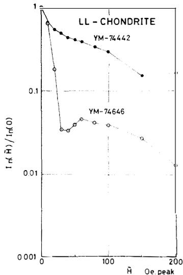
Fig. 6a. AF-demagnetization curves of NRM intensity for LL-chondrites.
