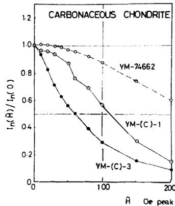
Fig. 1a. AF-demagnetization curves of NRM intensity for carbonaceous chondrites.
