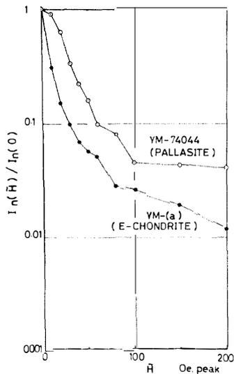
Fig. 7a. AF-demagnetization curves of NRM intensity for an E-chondrite and a pallasite.
