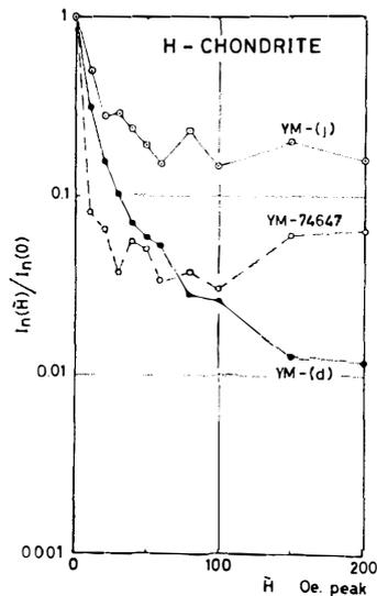
Fig. 4a. AF-demagnetization curves of NRM intensity for H-chondrites.
