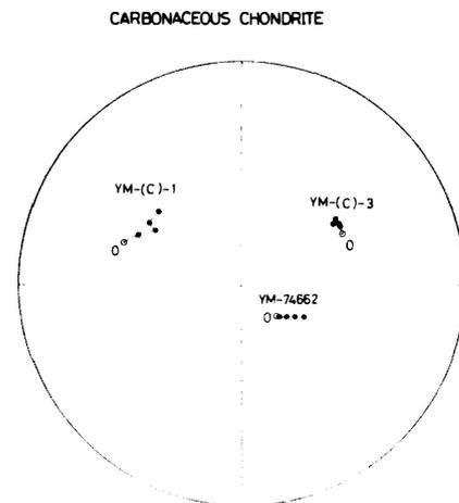
Fig. 1b. AF-demagnetization curve of NRM direction for carbonaceous chondrites.
