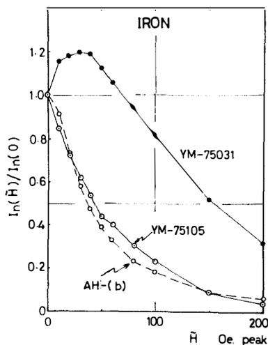
Fig. 3a. AF-demagnetization curves of NRM intensity for iron meteorites.
