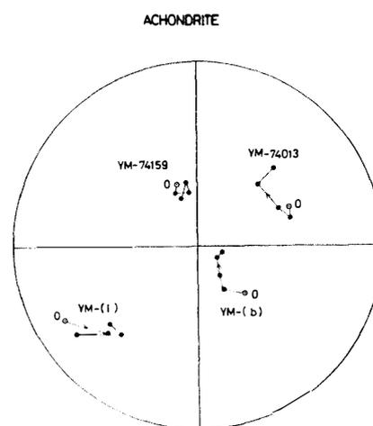
Fig. 2b. AF-demagnetization curves of NRM direction for achondrites.
