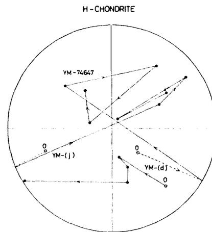
Fig. 4b. AF-demagnetization curves of NRM direction for H-chondrites. (Dotted lines are in the opposite hemisphere).
