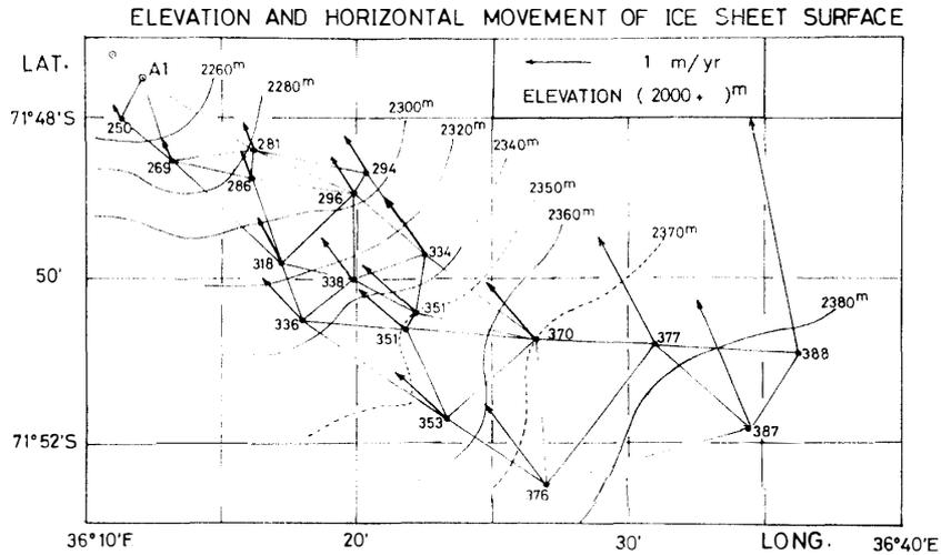
*Fig. 7. Horizontal movement and elevation of ice sheet surface near the Yamato Mountains.*
