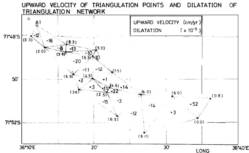
*Fig. 8. Upward velocity of the ice sheet surface and dilatation of the triangulation network near the Yamato Mountains.*
