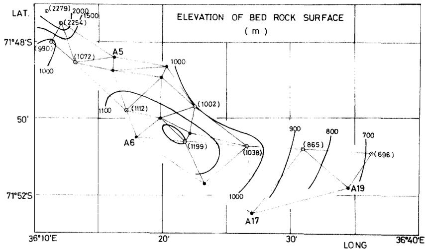
Fig. 9. Elevation of bedrock surface beneath the triangulation network.
