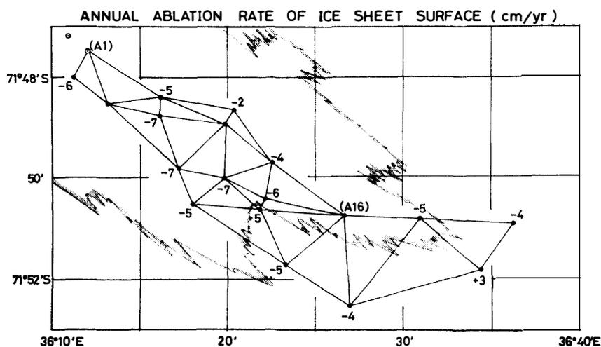
Fig. 10. Annual ablation rate of ice sheet surface over the triangulation network area near the Yamato Mountains (cm/year).
