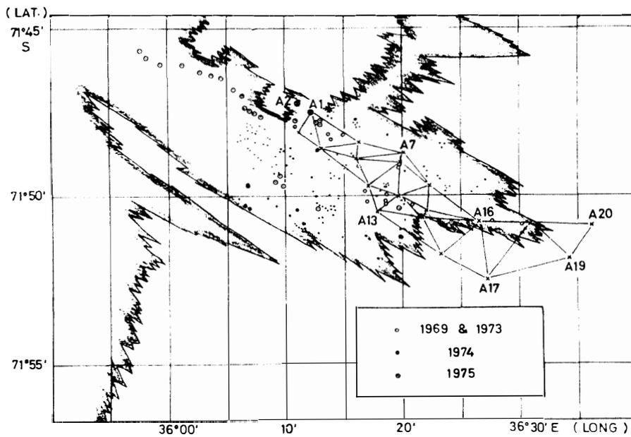
Fig. 6. Distribution of the Yamato meteorites in the southeastern corner of the Meteorite Ice Field, and the triangulation networks for measuring the ice sheet surface movement.
