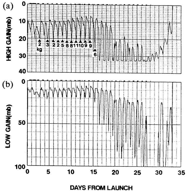
Fig. 8. Pressure gauge output in high gain mode (a) and low gain mode (b). Abscissas are time from launch, and ordinates are pressure in mb. The filled triangles and numbers below them in (a) show time and amount of ballast casting, respectively. Tip marks at the top of each panel show the time of position data acquisition.
