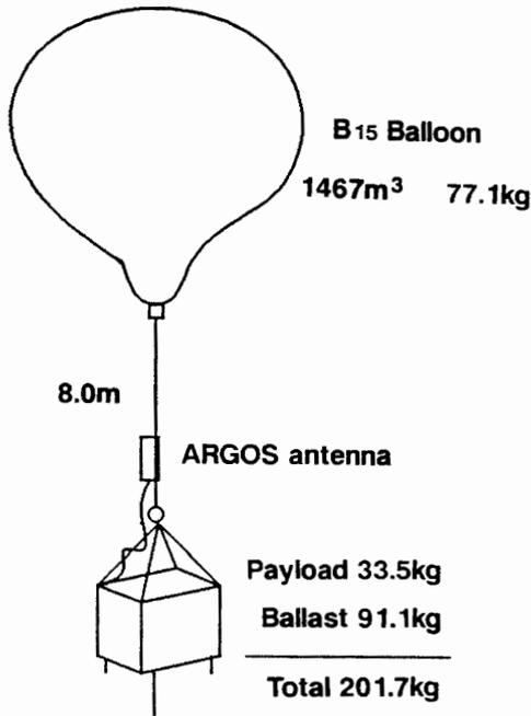
Fig. 1. Launching configuration of JARE-30's PPB.
