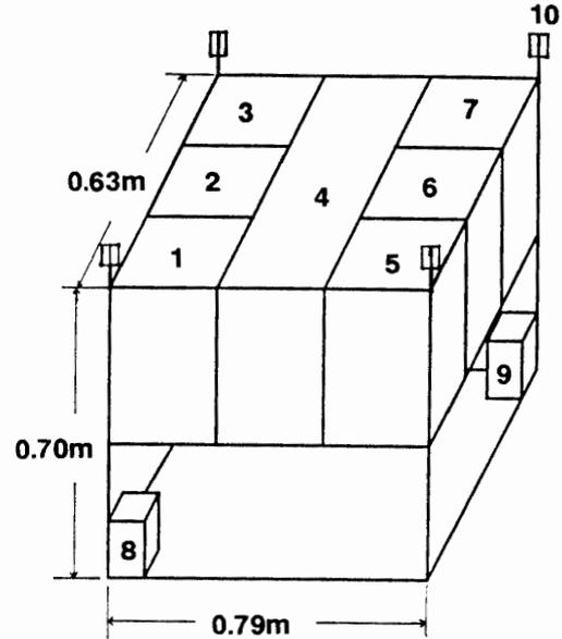
Fig. 2. Payload configuration of JARE-30's PPB. 1: pressure gauge; 2: Li battery 1; 3: ARGOS telemeter; 4: ballast; 5: command receiver; 6: Li battery 2; 7: electric circuits; 8: FM transmitter 1; 9: FM transmitter 2; 10: solar battery cell.
