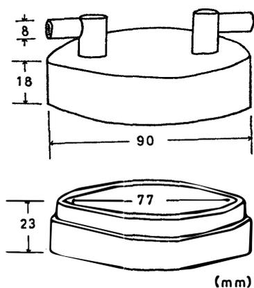
Fig. 2. Plastic chamber for measurement of carbon dioxide evolution rate.
