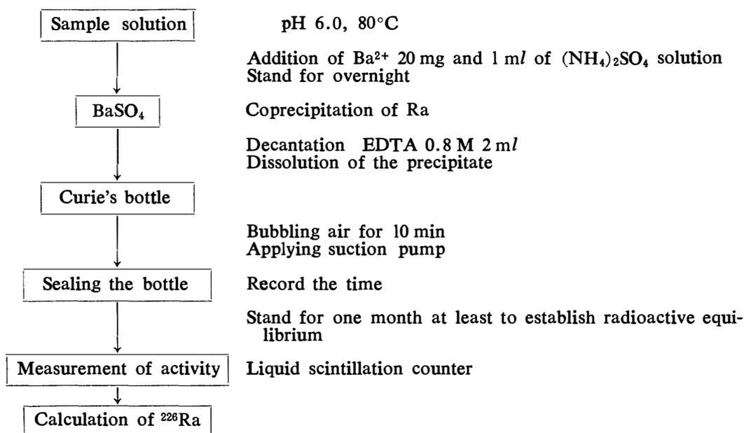
pump. The bottle was then sealed at the two branches under a reduced pressure and the time of sealing was recorded as the initiation time of Rn generation.
