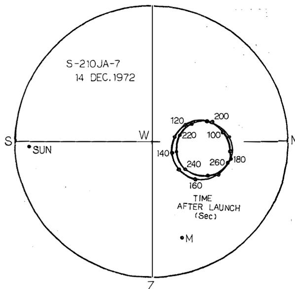
Fig. 3. The orientation of the rocket axis described on a stereographic net for the period between 90 and 260 s after the launching.
