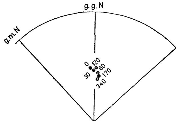
Fig. 3. Change in the direction of the remanent magnetization with the demagnetization by alternating magnetic field.
