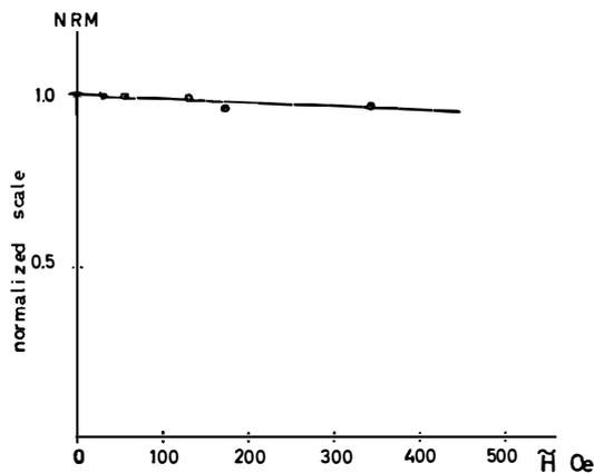
Fig. 2. Change in the intensity of the remanent magnetization with the demagnetization by alternating magnetic field.
