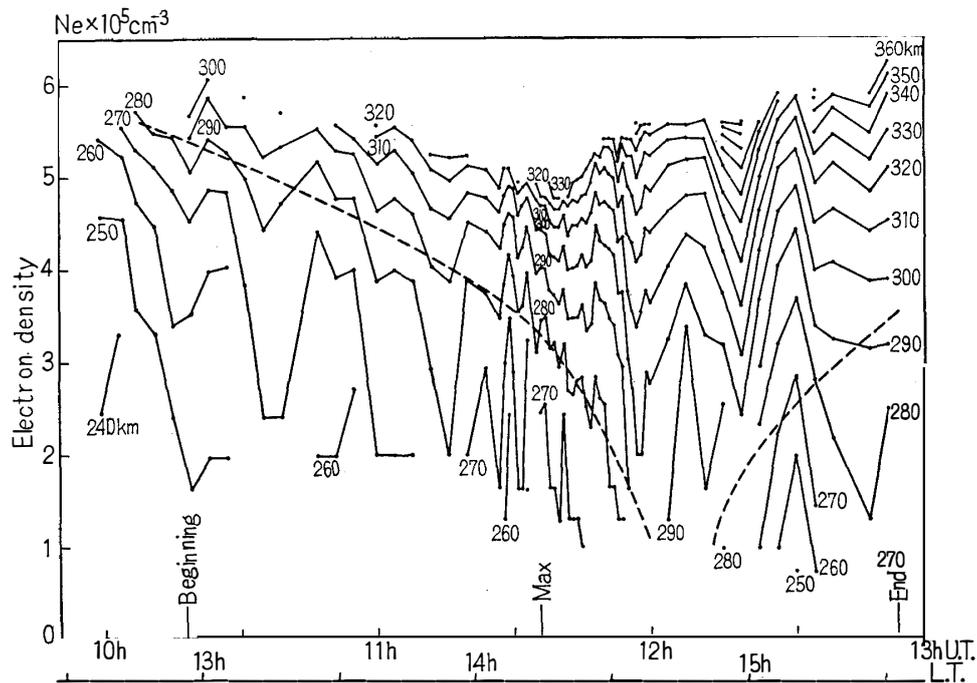
Fig. 7. Variation of the electron density  $N$  at various true heights during the eclipse on August 11, 1961, at Syowa Base.
