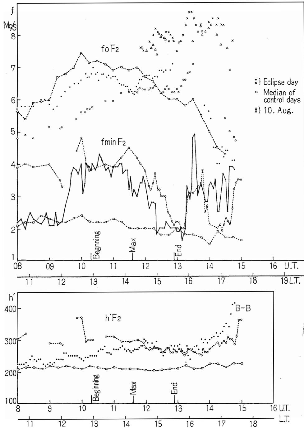
Fig. 3. Observational values of  $f_oF_2$ ,  $f_{min}F_2$ , and  $h'F_2$  during the eclipse on August 11, 1961, at Syowa Base.
