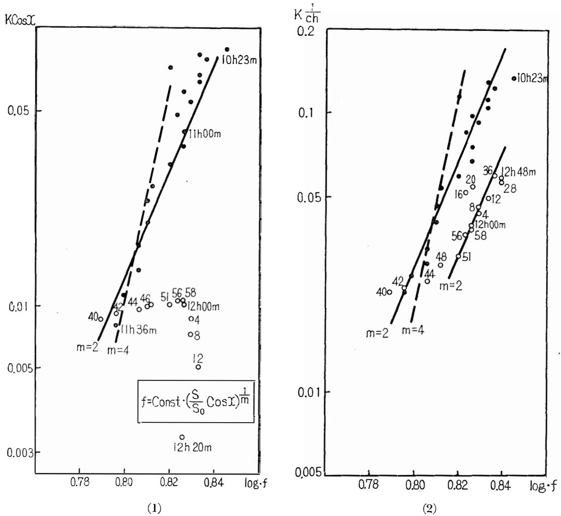
Fig. 5. Relation between  $\log f$  and  $\log K \cos X$  or  $\log K_1/ch$  for the F2 layer ( $m=2$ , slope of the straight line for attachment and  $m=4$ , that for recombination).
