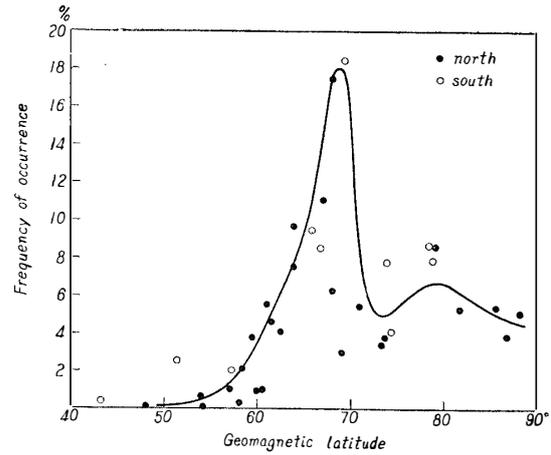
Fig. 2. Percentage hourly frequency of occurrence of blackouts for the whole period plotted against geomagnetic latitude.
