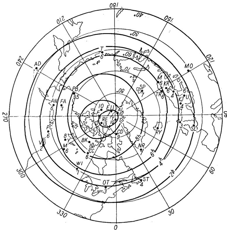
Fig. 6. Isochrons in local time of maximum frequency of occurrence of blackouts for the whole period shown on polar geomagnetic coordinates.
