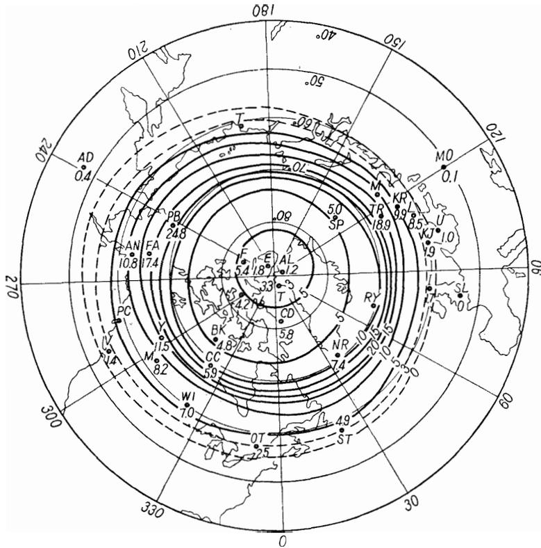
Fig. 4. Amplitude of diurnal variation of frequency of occurrence of blackouts for the whole period shown on polar geomagnetic coordinates.
