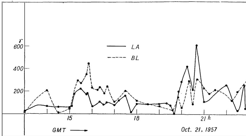
Fig. 9. Horizontal disturbance force at different stations (Bay-type variation, local day time).
