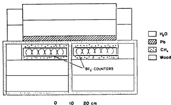
(A) Geometry of neutron pile.
