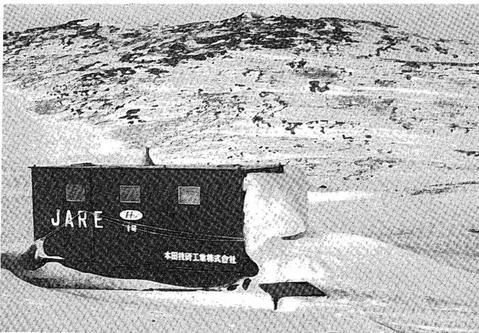
Photo. 5. The all-plastic caboose in Antarctic field (prepared and presented by Honda Giken Kōgyō Co.). The upper half of its chimney was not attached in this photograph.
