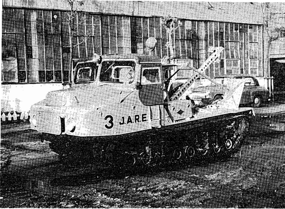
Photo. 3. Gasoline type snow-wrecker (prepared by the Komatsu Manufacturing Co. for the first expedition).
