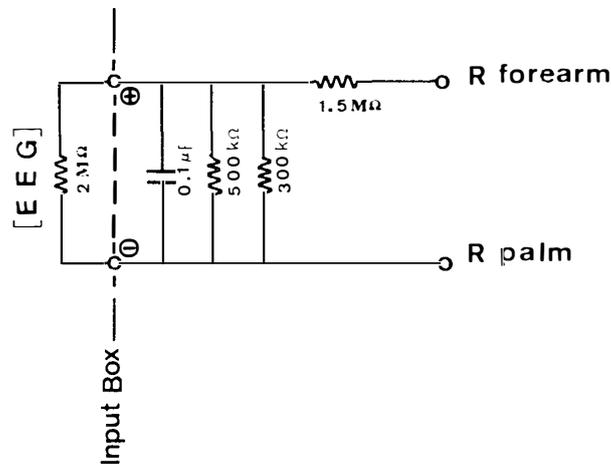
Fig. 1. Circuit placed between the subject and input box for recording skin potential reflex (SPR).
