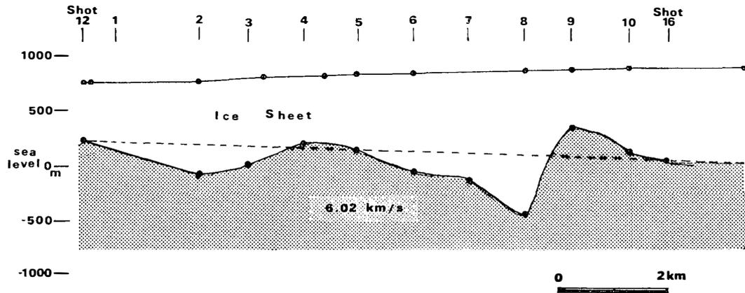
Fig. 6. Upper crustal structure revealed in the experiment. Surface elevation is after NARUSE and YOKOYAMA (1975).
