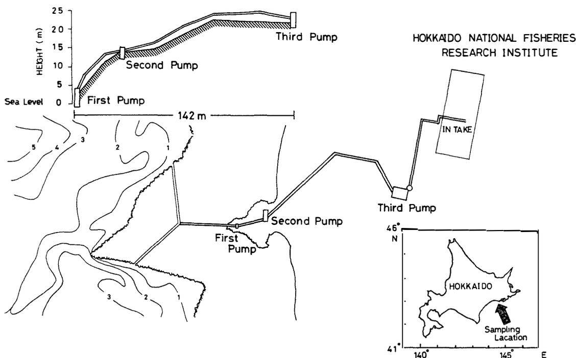
Fig. 1. Seawater system at the Hokkaido National Fisheries Research Institute, Kushiro, Hokkaido, Japan. Numbers along the contour lines indicate the depth of bottom. The top left portion indicates a vertical height of three pump stations in relation to the sea level. The total length from the first to third pump stations was 142 m. Inserted map indicates a sampling location.
