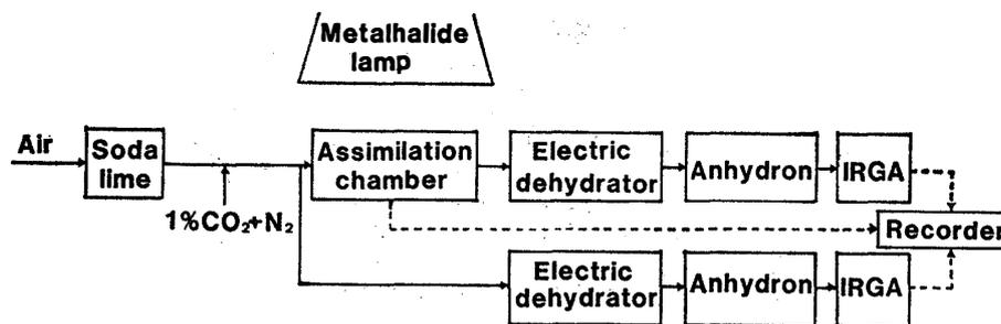
Fig. 2. The measurement system of net photosynthesis and dark respiration ( $\text{CO}_2$  uptake) in the laboratory on the research ship *SHIRASE* in the Antarctic and at Waseda University in Japan.
