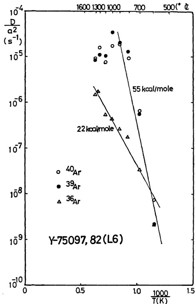
Fig. 4. Arrhenius plot for the sample Y-75097,82.
