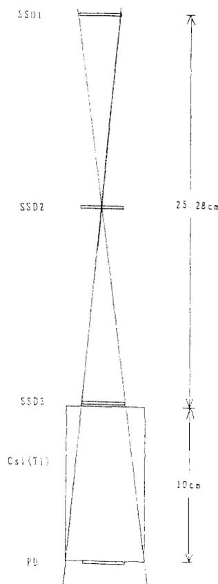
Fig. 2. The cosmic ray telescope consists of 3 SSDs and a CsI(Tl) viewed by a silicon photodiode triggered by coincidence with the 3 SSDs. This instrument named as D2 is one of three detectors on PPB #6.
