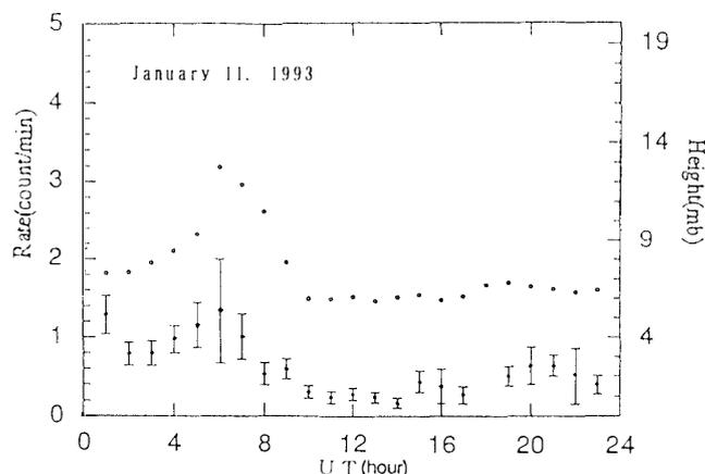
Fig. 3. One day variation of proton counting rate for January 11th marked as closed circles, and the balloon altitude in mb marked as open circles.
