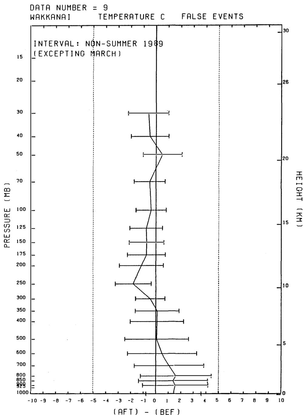
Fig. 1. Mean temperature difference over Wakkanai, Japan before and after randomly selected "false events" in winter (November–March) in 1989. The right-hand side vertical axis represents the geopotential height for each pressure level shown on the left-hand side axis.
