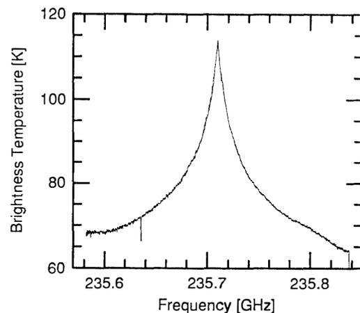
Fig. 2. Ozone emission line observed at the Nobeyama Radio Observatory. The integration time was 200 seconds. Frequency resolution was 0.3 MHz. Sky temperature was approximately coincided with liquid nitrogen temperature varying the elevation angle. The elevation angle was 40 degrees when this data was taken.
