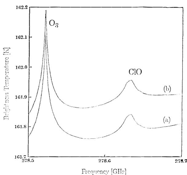
Fig. 3. Simulated ClO emission line. The U.S. standard atmosphere is assumed. (a) the standard ClO is used. (b) the ClO concentration measured by DE ZAFRA *et al.* (DE ZAFRA *et al.*, 1989) is used.
