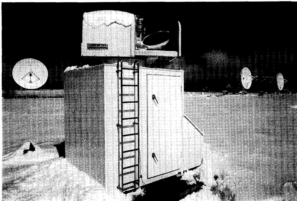
Fig. 4. *The University of Tokyo-Nobeyama Radio Observatory 60-cm Galactic Survey Telescope.*
