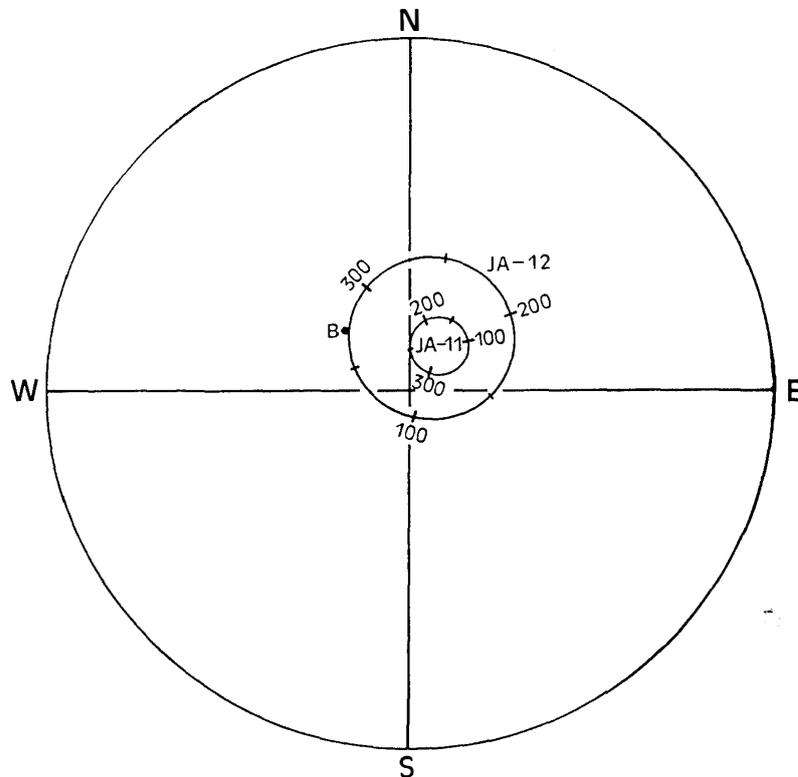
Fig. 3. Absolute orientations of two sounding rocket axes on the Wulf's stereographic projection.
