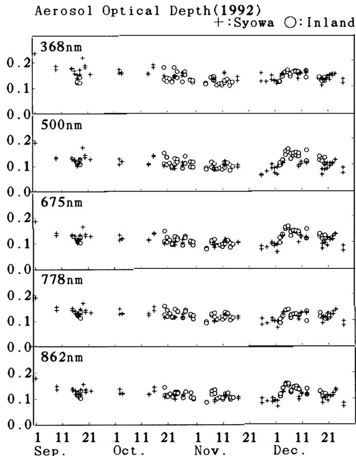
Fig. 5. Aerosol optical depths from September to December 1992 observed by the Syowa fixed instrument and the portable inland one (daily maxima and minima are shown). The September data are results of simultaneous observations at Syowa.
