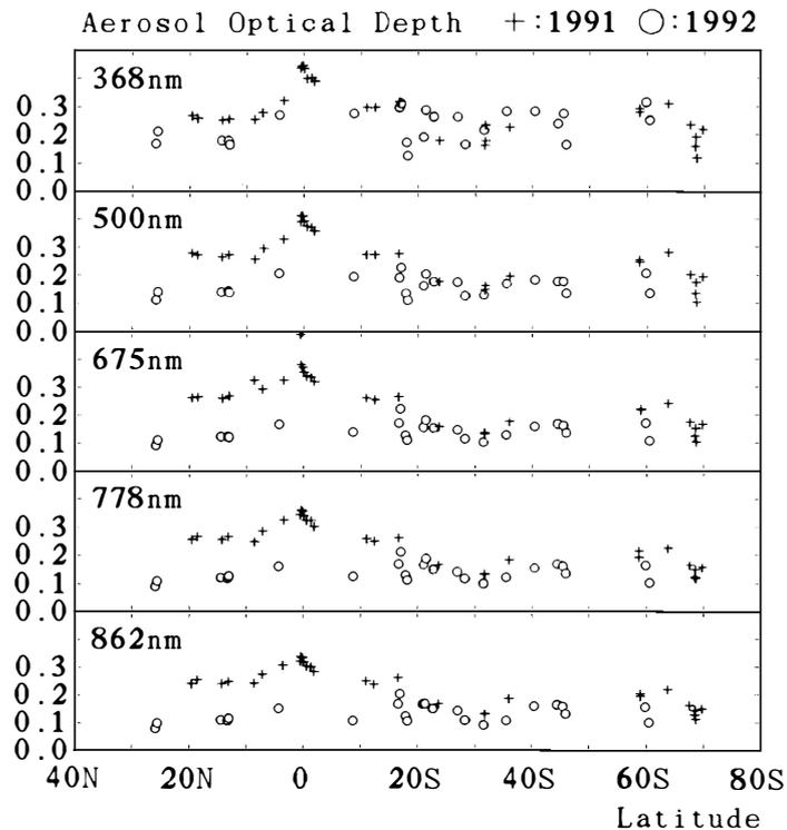
Fig. 3. Aerosol optical depth of 1991 and 1992 from onboard observations at each wavelengths (All data of  $M < 3$  are used).
