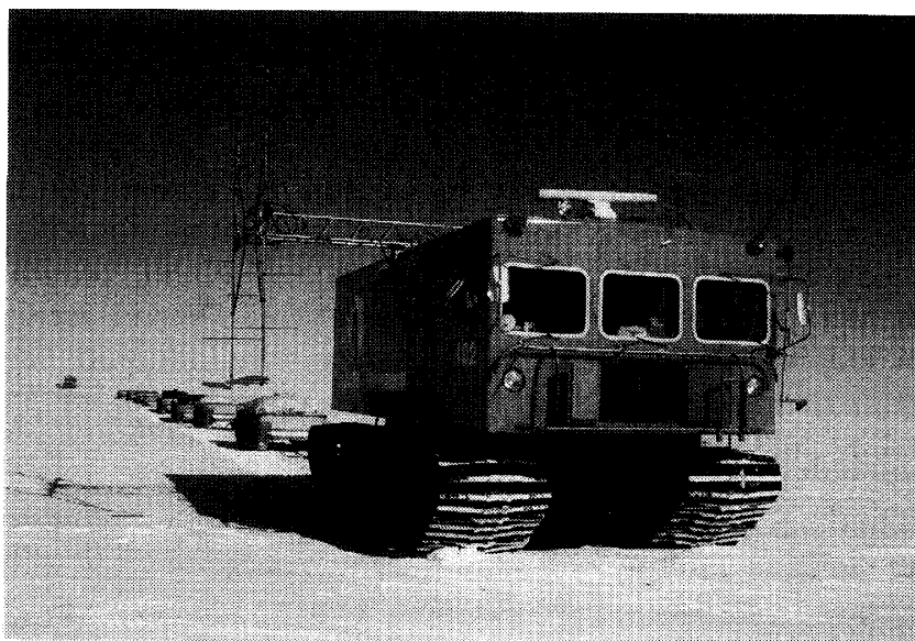
Fig. 1. Oversnow vehicle with the antennas of the radio echo sounder on the roof.
