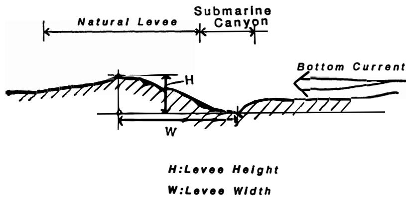
Fig. 2. A transversal profile of the submarine canyon on the continental rise. Bottom current is parallel to the contour. The levee height ( $H$ ) is measured from main channel floor to the top of the levee ridge (see text).
