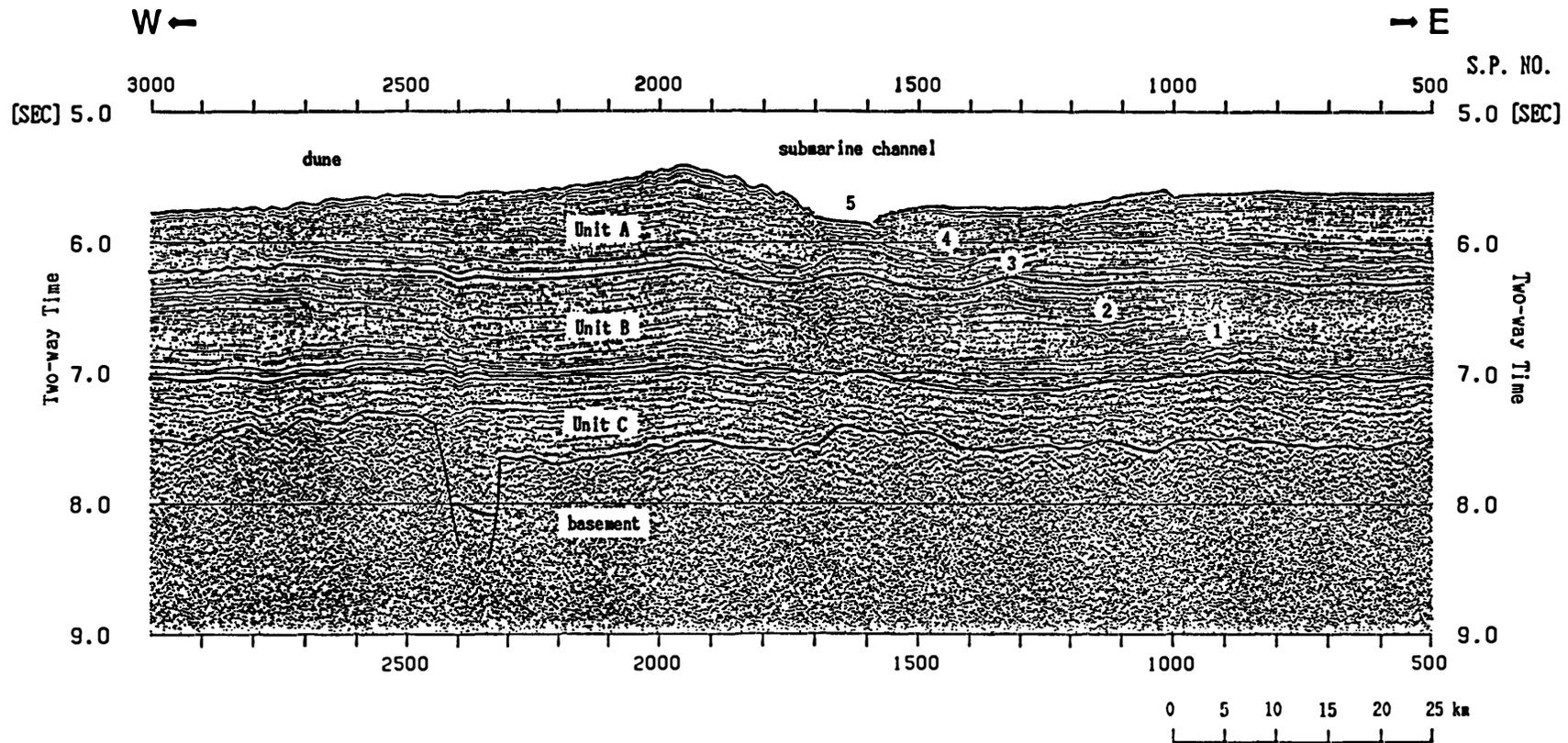
Fig. 4. Seismic reflection profile from the Amundsen Sea (YAMAGUCHI *et al.*, 1988). Natural levee develops to the left (west) of the canyon. Numbers in white circles show the migration direction of leveed channels.
