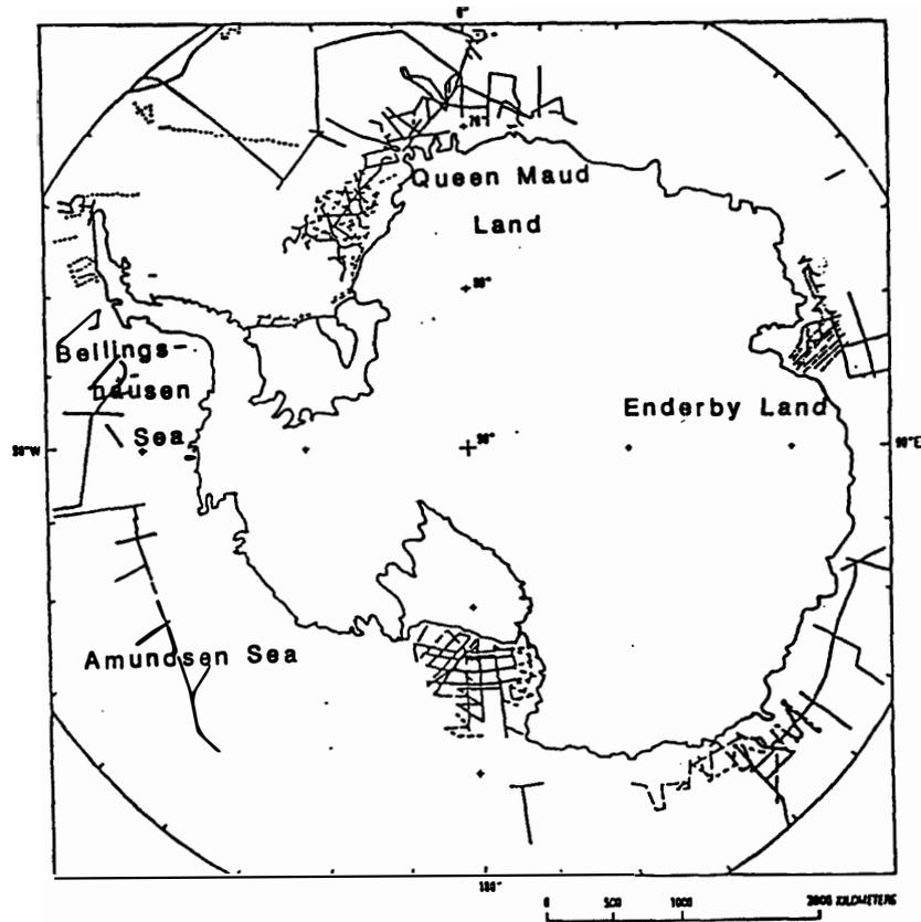
Fig. 1. Locality map of seismic reflection lines in the Southern Ocean.
