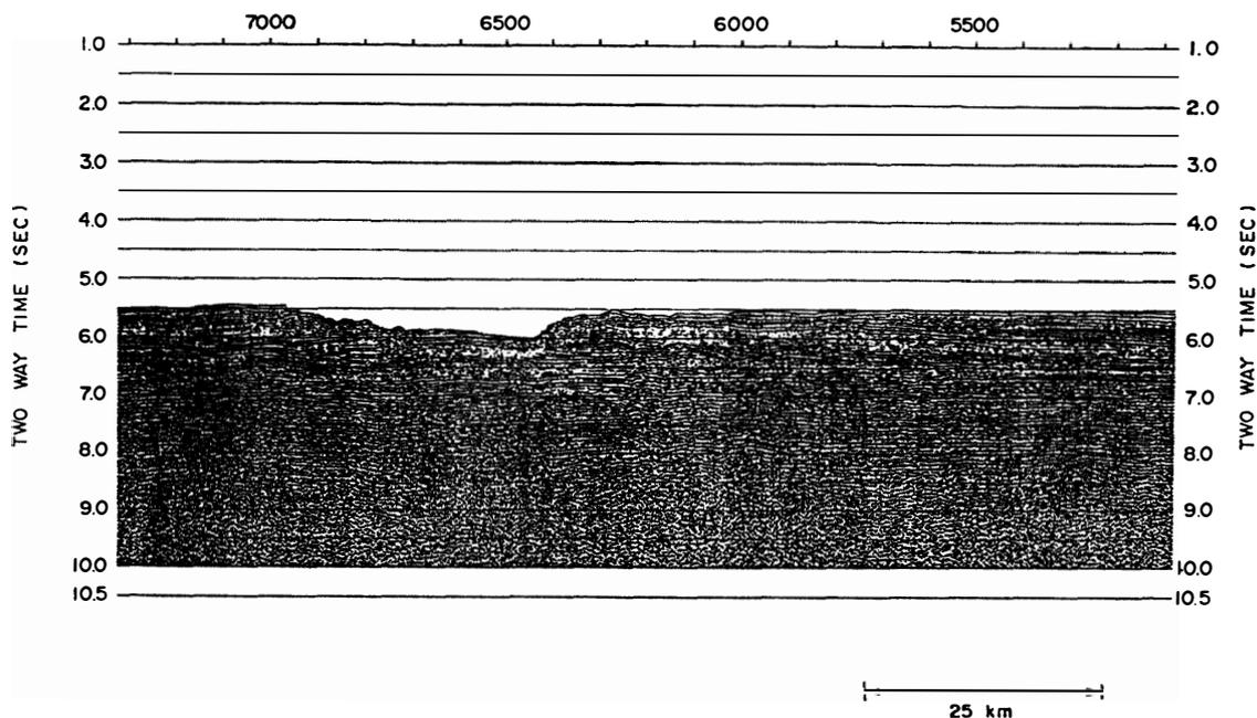
Fig. 5. Seismic reflection profile from offshore of Queen Maud Land (SAKI *et al.*, 1987). A large-scale canyon is observed with slightly higher levee on the left side (west) of the canyon.
