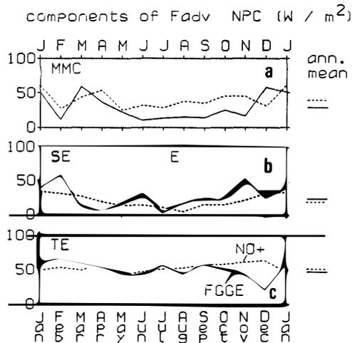
Fig. 4. Components of the advective term of energy budget for the north polar cap. The unit is  $W m^{-2}$ . (a) Mean meridional circulation, (b) stationary eddies, (c) transient eddies.
