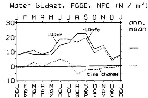
Fig. 7. Components of monthly water budget of the north polar cap resulting from FGGE data. The unit is  $W m^{-2}$ . The horizontal lines at the right margin show the annual mean values. Dotted line: local time change; Dashed line: advection; Solid line: precipitation minus evaporation.
