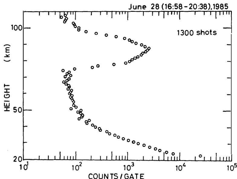
Fig. 1. Vertical profile of echo signals (A-scope) by accumulating the returns of 1300 laser shots on June 28 (1658–2038 LT or 1358–1738 UT), 1985. The height resolution is 1 km.
