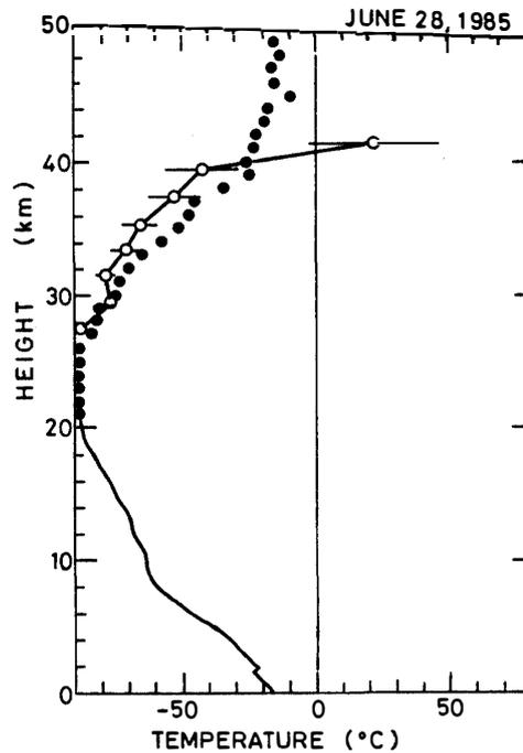
Fig. 2. Comparison of the temperature profile by lidar measurements ( $\circ$ ) with that by rocket sounding (MT-135JA) ( $\bullet$ ). The solid curve below 21 km indicates the temperature profile by meteorological sonde sounding.
