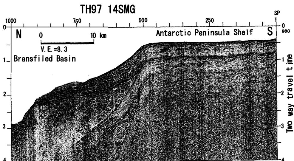
Fig. 13. Detailed color coded multichannel seismic reflection profile of 14SMG at the western part of eastern Bransfield Basin.
