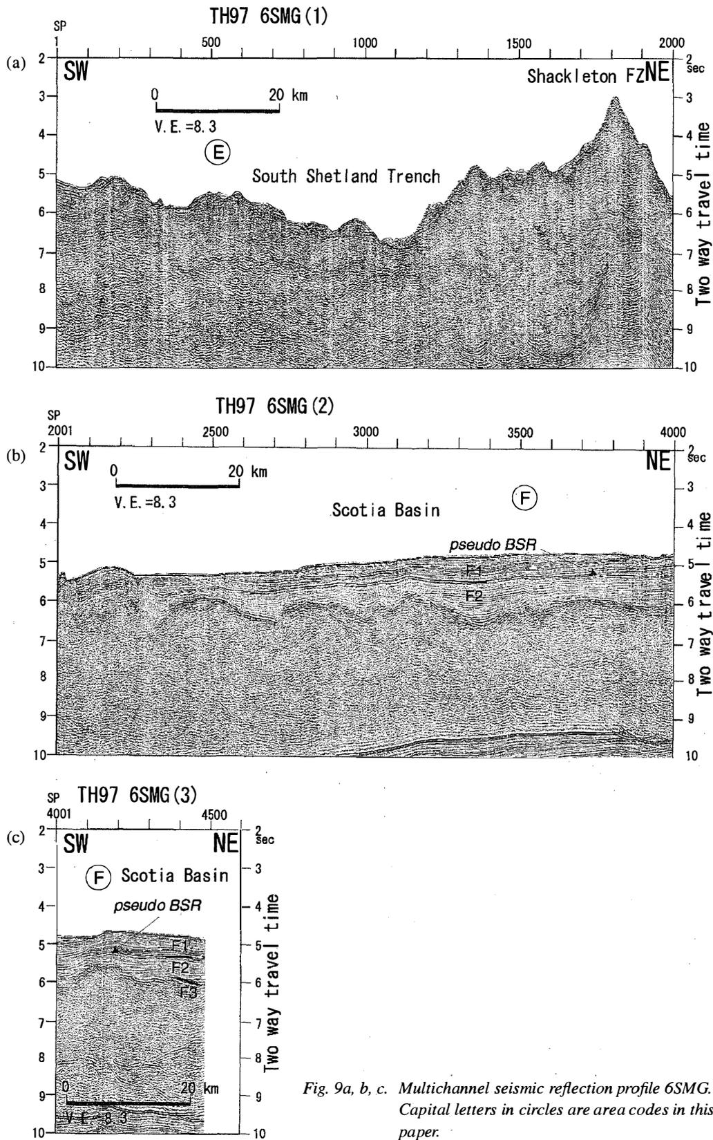
Fig. 9a, b, c. Multichannel seismic reflection profile 6SMG. Capital letters in circles are area codes in this paper.
