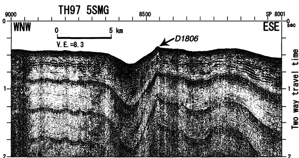
Fig. 14. Detailed color coded multichannel seismic reflection profile of 5SMG at the D1806 dredge site, southwest of Elephant Island.
