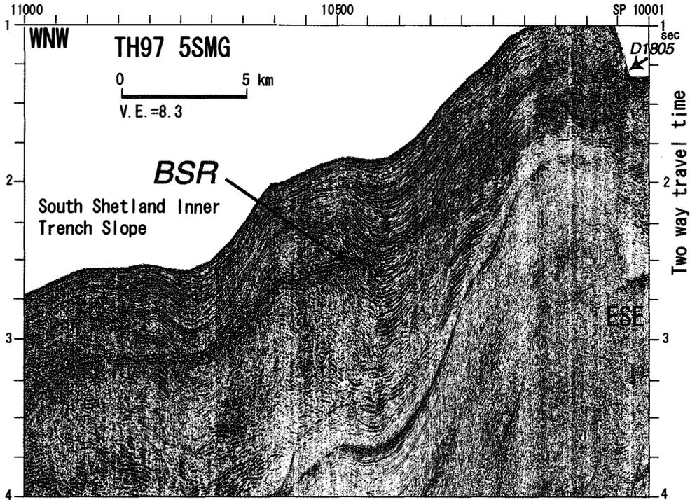
Fig. 15. Detailed color coded multichannel seismic reflection profile of 5SMG at the continental slope. Note the distinct BSR (Bottom Simulating Reflector).
