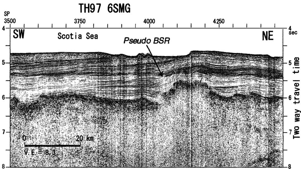
Fig. 16. Detailed color coded multichannel seismic reflection profile of 6SMG at Scotia Basin. Note the pseudo-BSR (Bottom Simulating Reflector).
