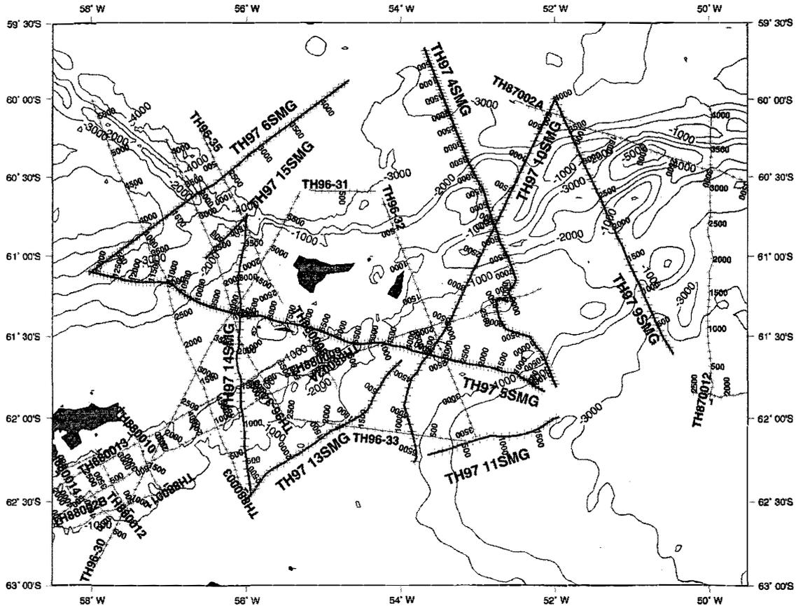
Fig. 6. Multichannel seismic reflection survey lines during the TH97 cruise. Thin lines are the TH87, TH88 and TH96 survey lines. The numbers along the survey lines are SP (Shot Point) numbers.
