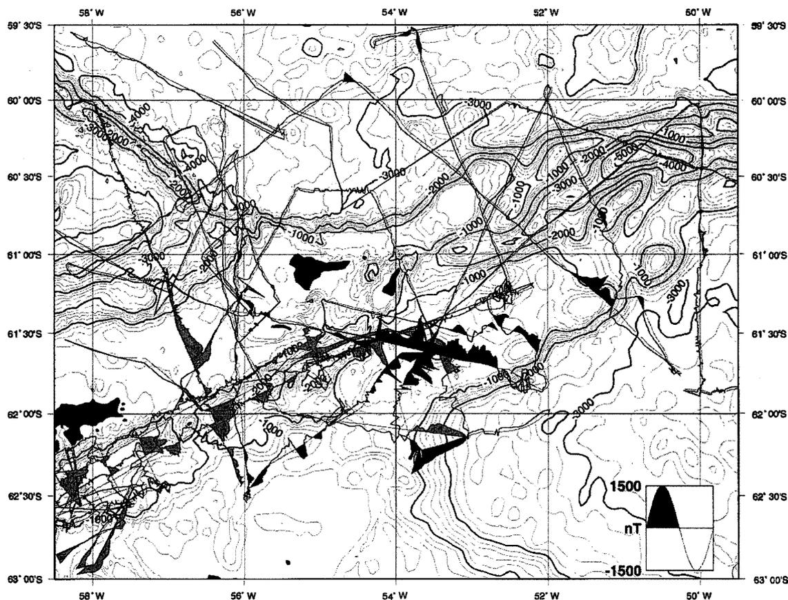
Fig. 5. Total magnetic anomaly profiles along the ship's track during the TH97 cruise at the northern margin of the Antarctic Peninsula. Gray profiles show previous JNOC cruise data during TH87, TH88 and TH96.
