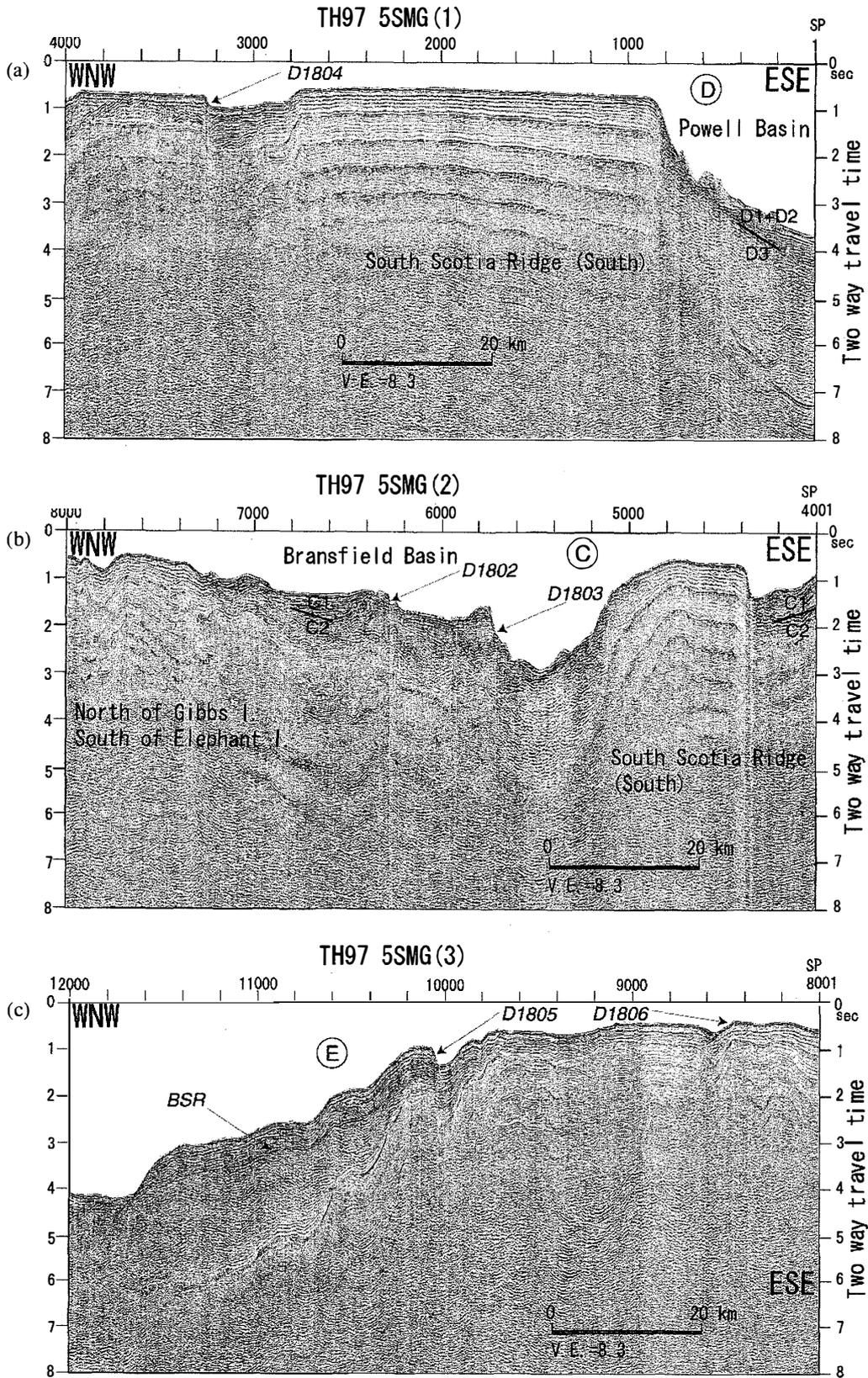
Fig. 8a, b, c. Multichannel seismic reflection profile 5SMG. Capital letters in circles are area codes in this paper:
