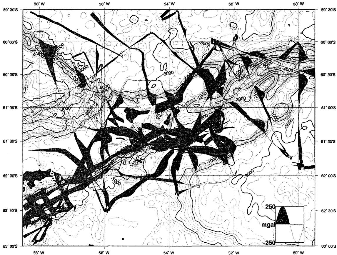
Fig. 4. Free-air gravity anomaly profiles along the ship's track during the TH97 cruise in the northern margin of the Antarctic Peninsula. Gray profiles show previous JNOC cruise data during TH87, TH88 and TH96.
