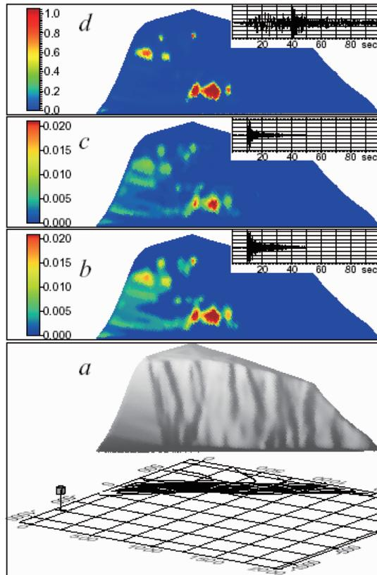
Fig. 9. Application of Newmark analysis to an avalanche prone area. Color bars show displacement in meters. Inserts show seismic time histories used in calculations.
