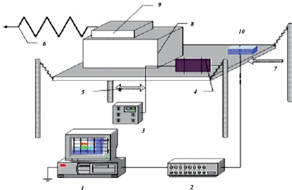
Fig. 10. A sketch of the installation for simulation of seismic vibration and its influence on snow shear strength. 1. Computer; 2. ADC; 3. Frequency regulator; 4. Vibrator; 5. Periodic oscillations; 6. Constant shear load; 7. Short impulse shock load; 8. Snow block; 9. Shear frame; 10. Seismic sensor (accelerometer). It is also possible to simulate static and dynamic normal loading.
