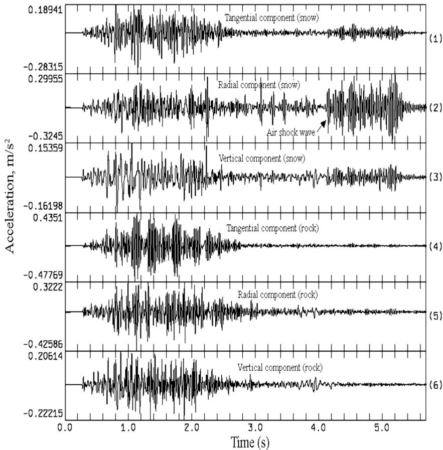
Fig. 4. An example of acceleration records for snow surface and underlying surface (rock). Snow cover depth and mean density at the measurement site are 0.8 m and  $260 \text{ kg/m}^3$  respectively.
