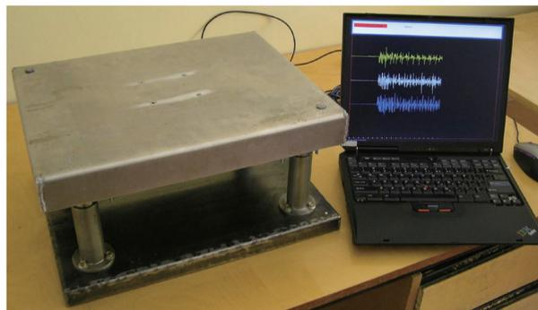
Fig. 11. The modernized shaking table.
