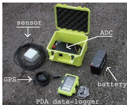
Fig. 3. Portable seismic station Cossack Ranger.
