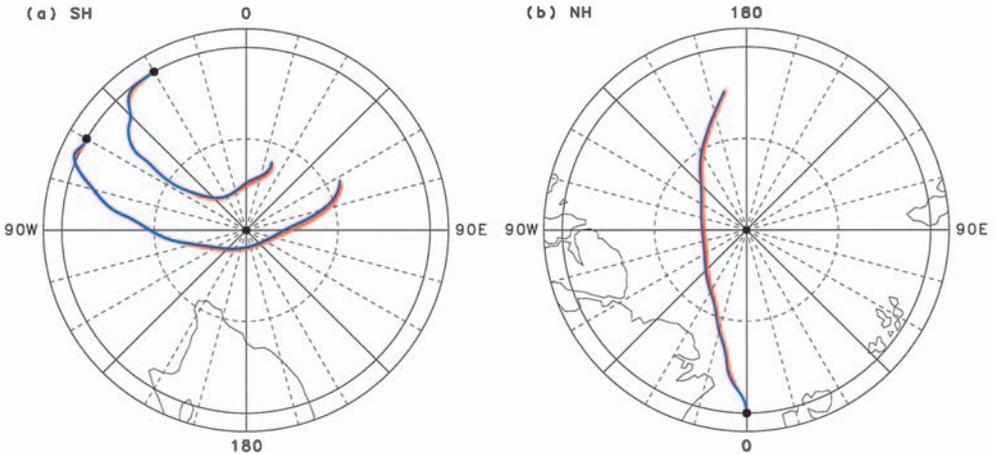
Fig. 7. Isentropic trajectories at 500 K, which passed (a) south of 87.5°S and (b) north of 87.5°N. Blue and red lines represent the trajectories calculated with the NIPR model and METEX, respectively. Solid circles show the initial positions. Solid and dashed latitude lines represent 80° and 85° latitudes, respectively.
