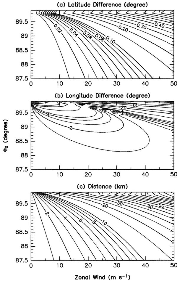
Fig. A1. (a) Latitude difference (degrees), (b) longitude difference (degrees), and (c) distance (km) between  $(\lambda_1, \phi_1, X_1, Y_1)$  and  $(\lambda_2, \phi_2, X_2, Y_2)$  as a function of zonal wind ( $\text{m s}^{-1}$ ) and  $\phi_0$  (degrees) for  $v=10 \text{ m s}^{-1}$ .
