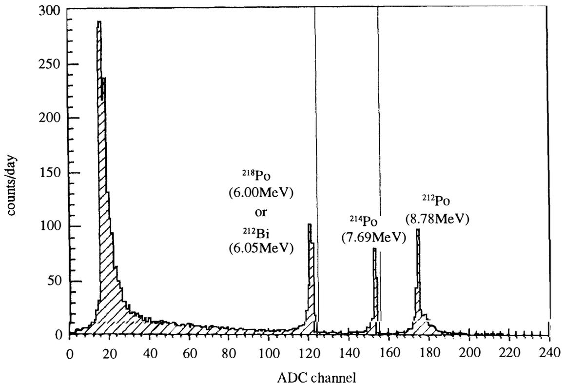
Fig. 2. A typical  $\alpha$ -spectrum from  $^{222}\text{Rn}$  and  $^{220}\text{Rn}$  daughters. This spectrum was obtained at SYO in October 1996. The vertical lines indicate the range of the ADC 125–156 channel. Signals in this range were used as the energy of  $\alpha$  particles from  $^{214}\text{Po}$  decay. The signals around ADC channel 20 indicate electric noise.
