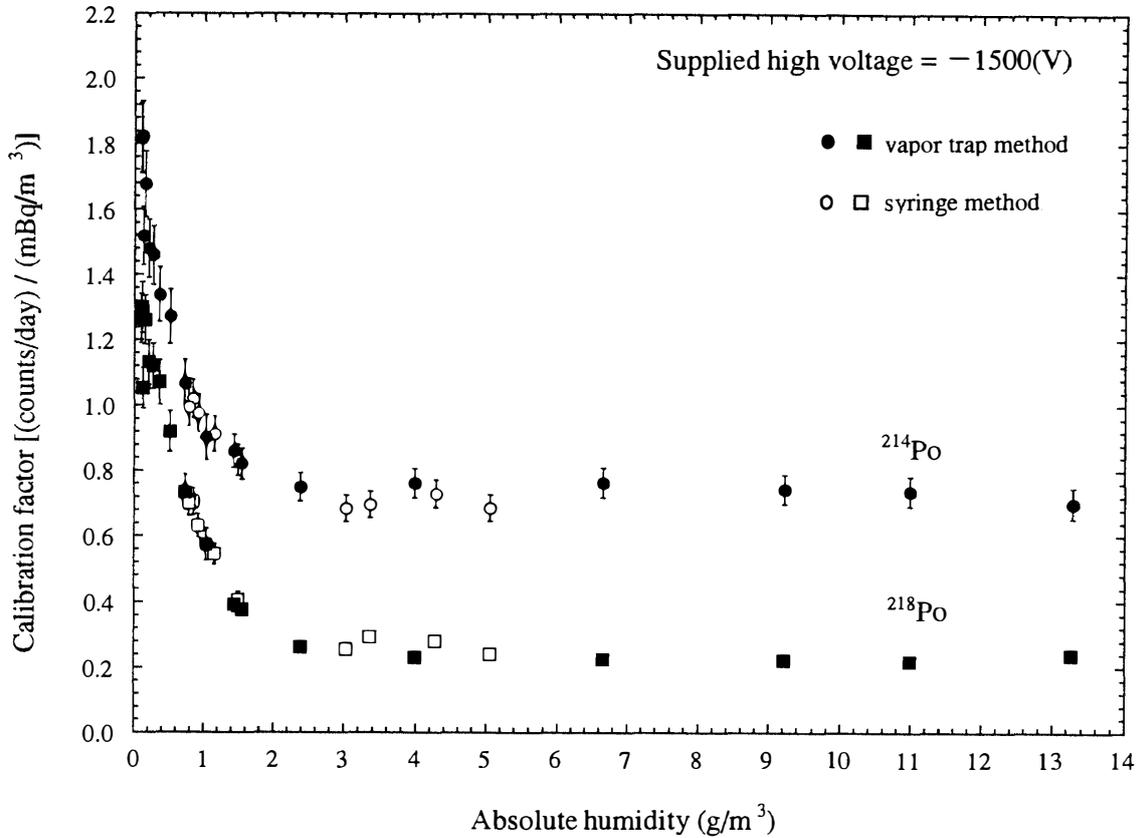
Fig. 5. Absolute humidity dependence on the calibration factors for the high sensitive atmospheric radon detector at supplied high voltage of  $-1500$  V.
