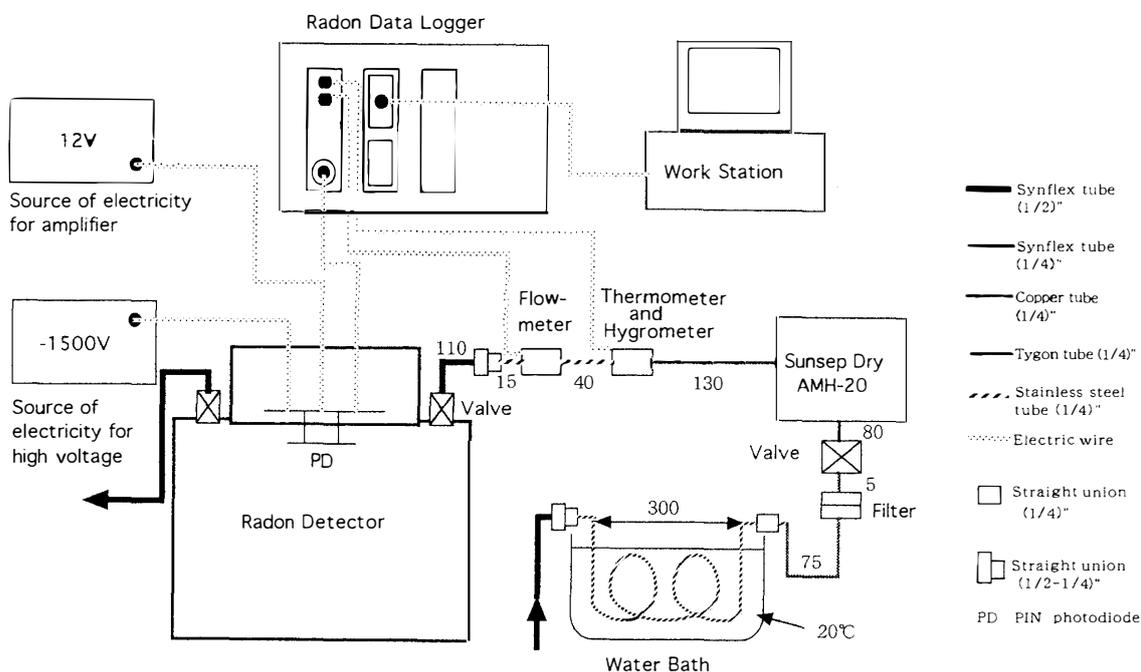
Fig. 6. A schematic diagram for the radon observation system at SYO. The total intake tube line is about 10 m long.
