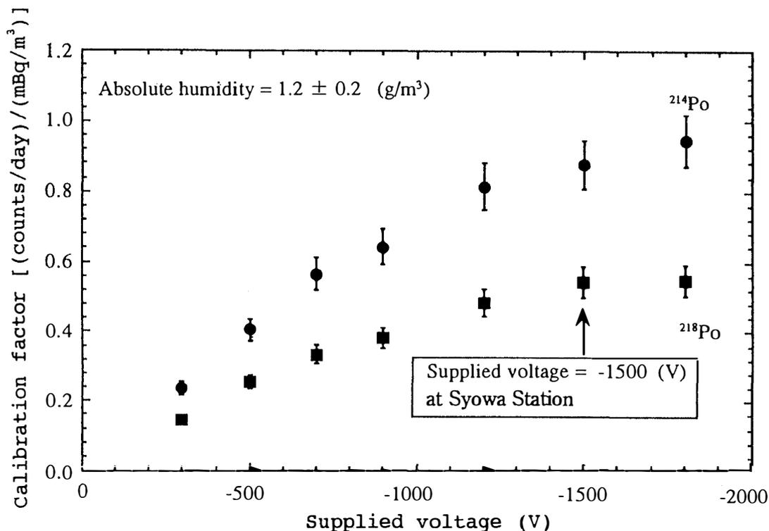
Fig. 4. High voltage dependence on the calibration factors for the high sensitive atmospheric radon detector at the absolute humidity of  $1.2 \pm 0.2$  (g/m<sup>3</sup>). The supplied high voltage was  $-1500$  V at SYO.
