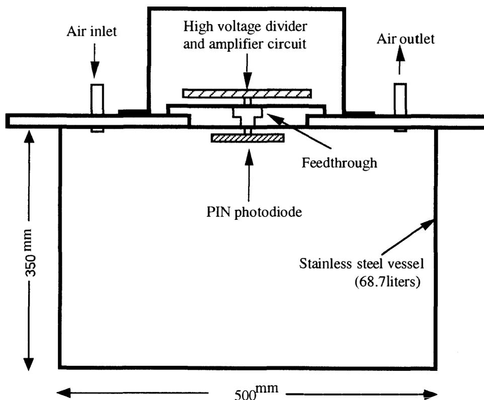
Fig. 1. A schematic view of a high sensitivity detector to measure the radon concentration in air.
