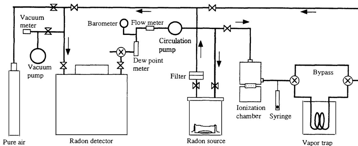
Fig. 3. A schematic diagram of the calibration system for high voltage dependence and humidity dependence measurement.
